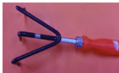
Floor groove cleaner for cattle sheds of Gaushala.
