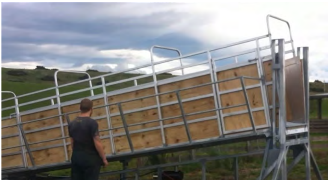
Height adjustable ramp fitted with motor compatible with all transporting vehicles of varying height.
