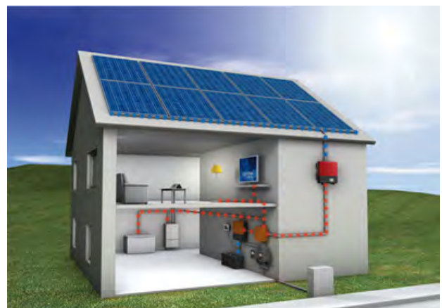
Rooftop grid connected solar system.
