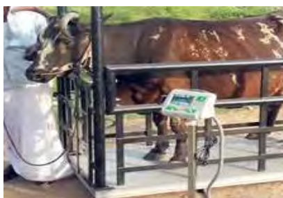
Heavy duty platform weight balance for measuring weights of animals at regular intervals to assess their health and well being.
