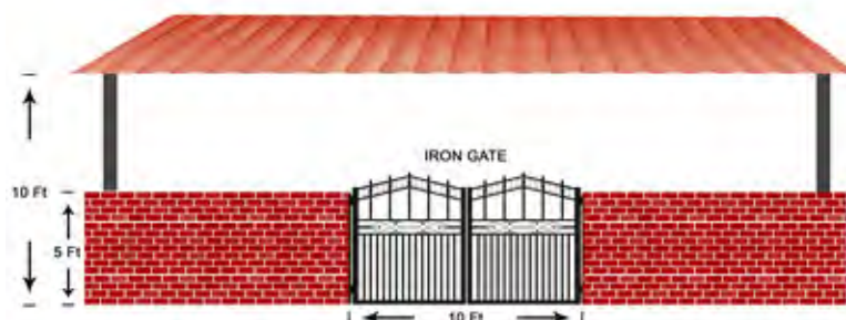
Construction details of animal examination area.
