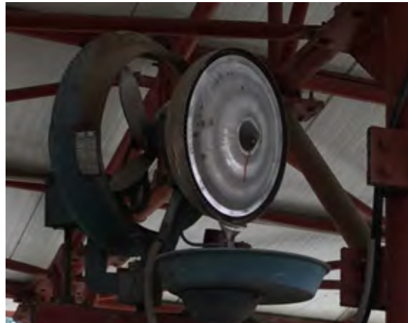
Picture of a fan fitted with fogger for keeping the temperature inside the shed low.
